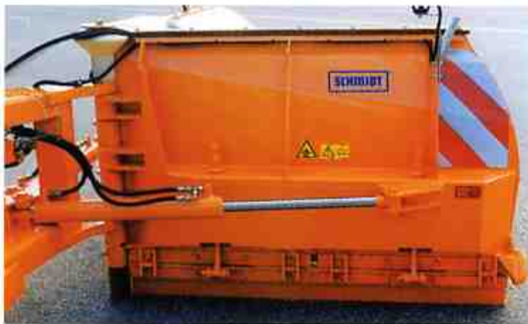
Robust hydraulic cylinders, a safety kickback system and the ideal blade profile.
