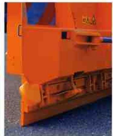
The automatic kickback system ensures safe operation in all plough forms
