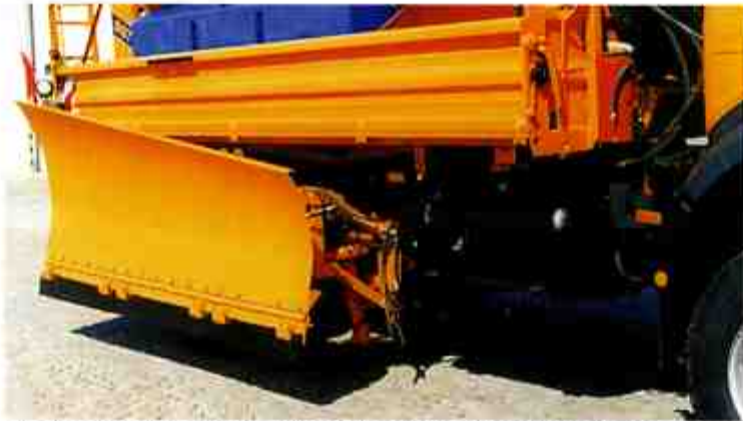
CPS 5.3 side-wing plough in transit position, with automatic safety latch
