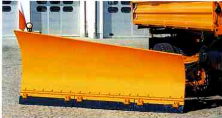
CPS 5.3 side-wing plough with „constant position“ kickback system
